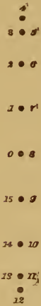
Fig. iv. Diagram of movement of wave-particle during one complete undulation of a distortional wave.
